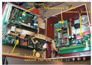
Software version is found on an IC on I/O board.
